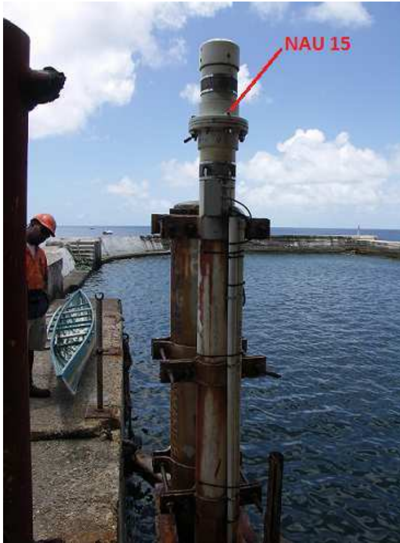
Figure 3 Nauru Tide Gauge with indications of NAU15 mark
