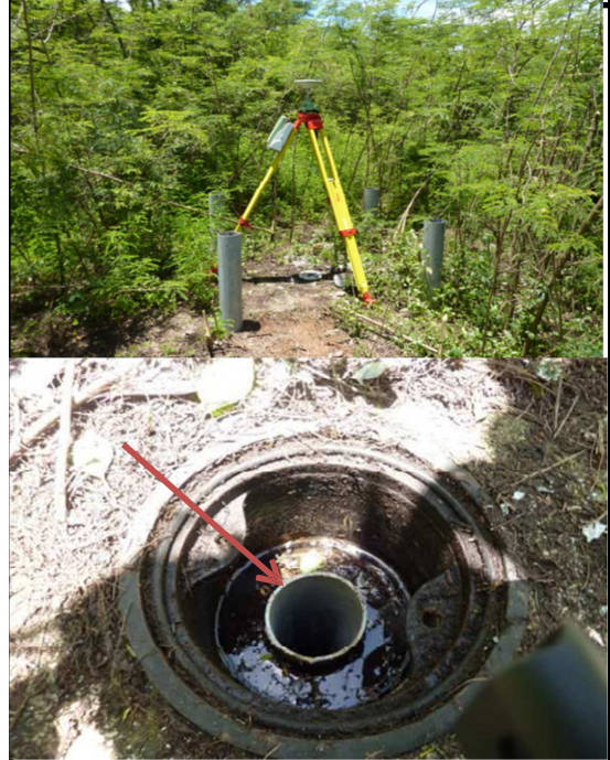
6 cm = elevation difference between ground level and PVC pipe top
