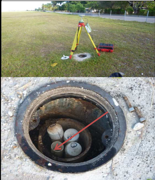
13,4 cm = elevation difference between ground level and PVC pipe top
