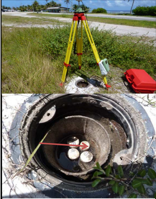
20 cm = elevation difference between ground level and PVC pipe top
