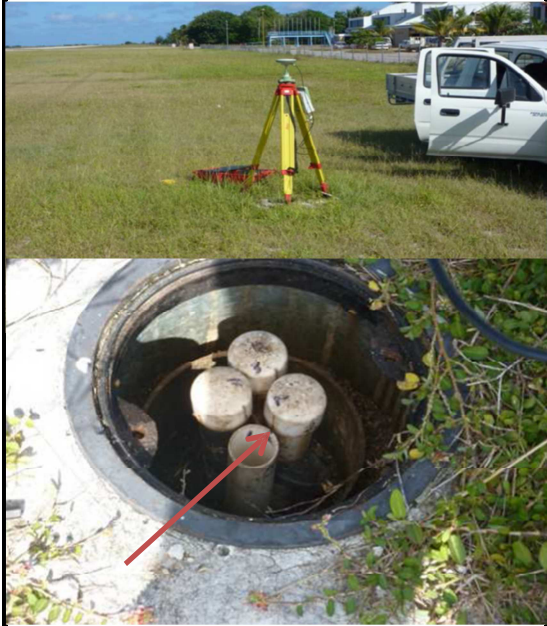
6,2 cm = elevation difference between ground level and PVC pipe top
