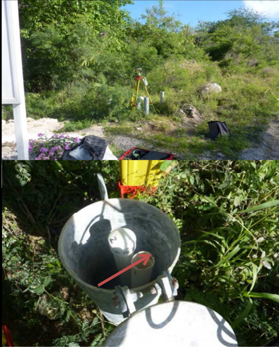
3 cm = elevation difference between external steel pipe top and PVC pipe top
