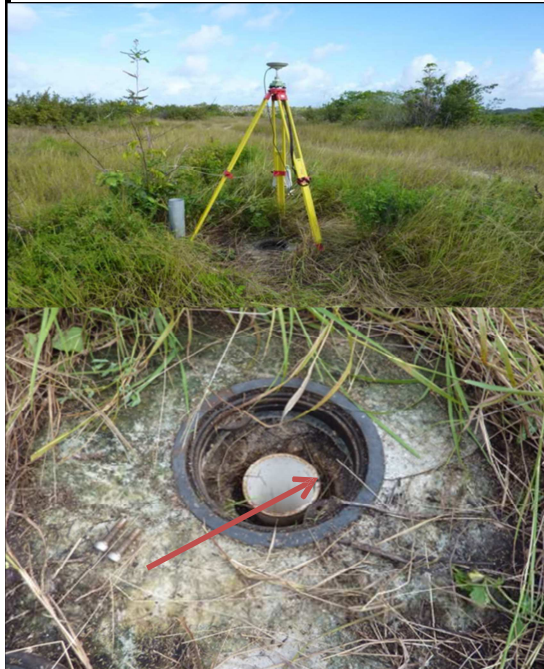
10 cm = elevation difference between ground level and PVC pipe top
