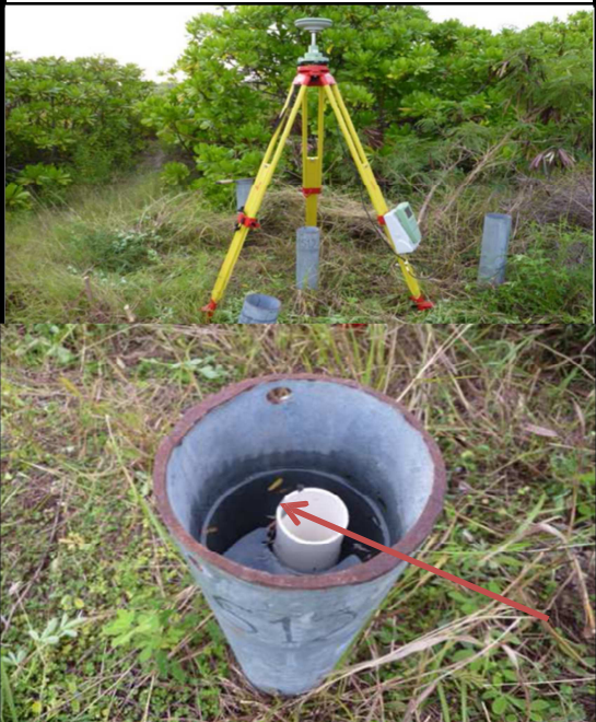
4 cm = elevation difference between external steel pipe top and PVC pipe top
