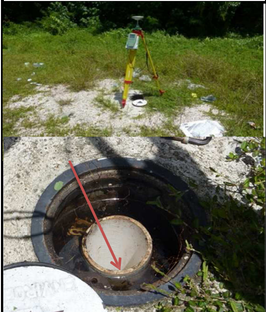
12 cm = elevation difference between ground level and PVC pipe top
