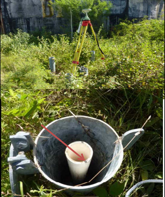
4,4 cm = elevation difference between external steel pipe top and PVC pipe top
