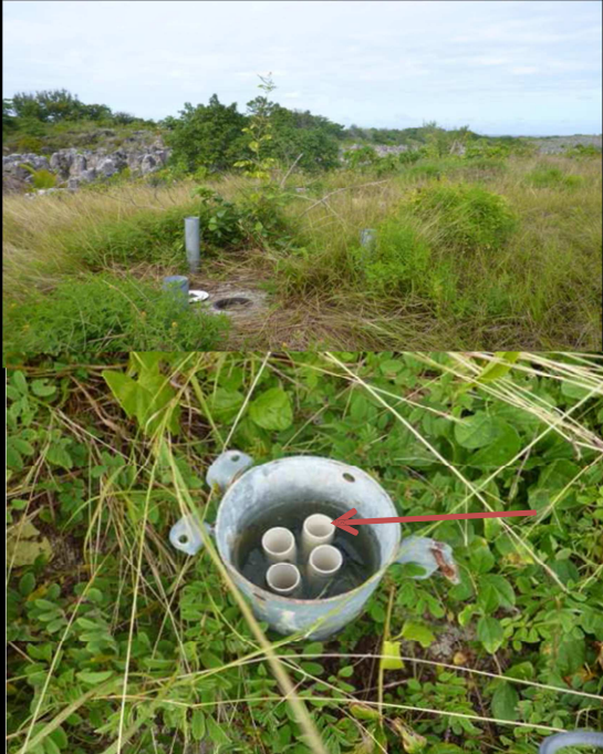
6,8 cm = elevation difference between external steel pipe top and PVC pipe top
