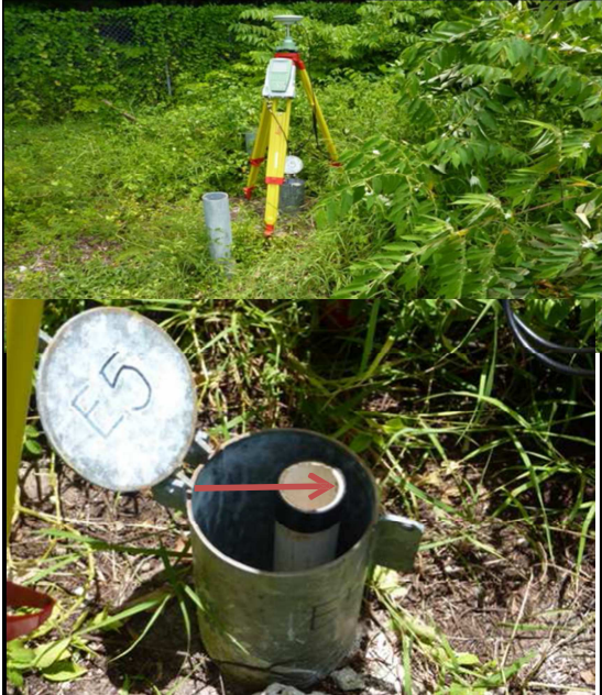
1 cm = elevation difference between external steel pipe top and PVC pipe top
