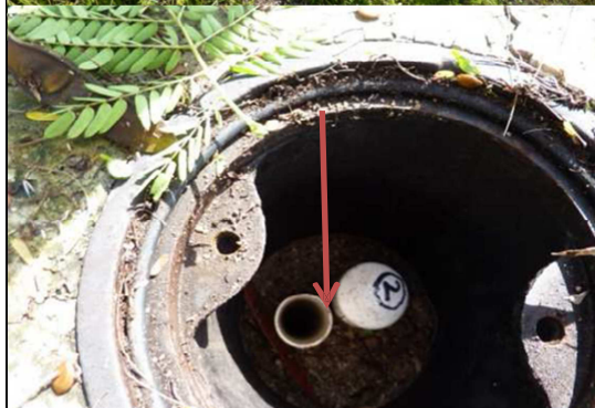
14,8 cm = elevation difference between ground level and PVC pipe top
